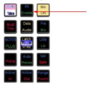
This opens a menu which allows selective enabling of mixer parameters for Write. Select {Faders} from the menu.
