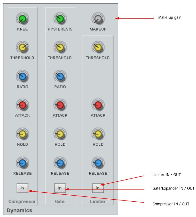
Each section has an independent IN / OUT control. All three may be active at the same time if required. The Fat Channel shows the transfer function of the dynamics control, plus gain reduction metering.
