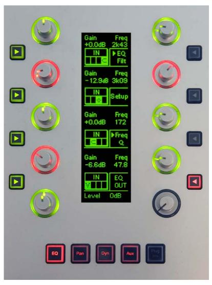
Once a signal path is on the Parameter Pad, you can control its fundamental signal processing with real time controls.
